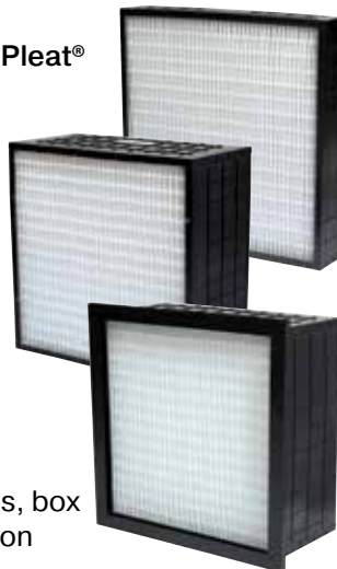
Adhesive beads bond the pleats into a rigid pack for even loading and complete media utilization.
